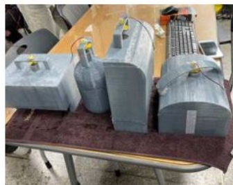
wave energy power plant designed by CAD and printed by 3D printer
